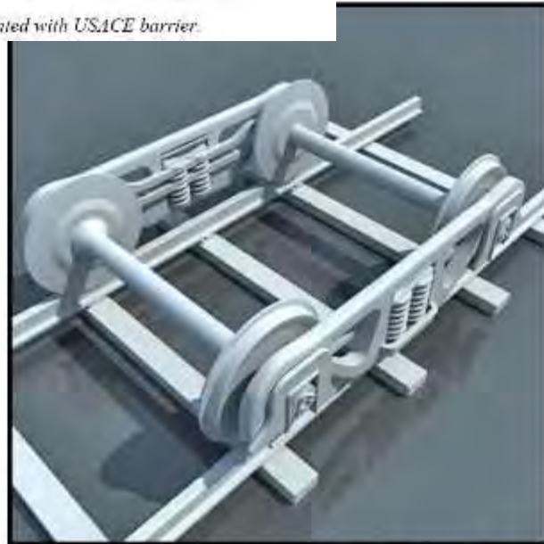
Figure 5: Conceptual wheel system for each barrier segment [4].
